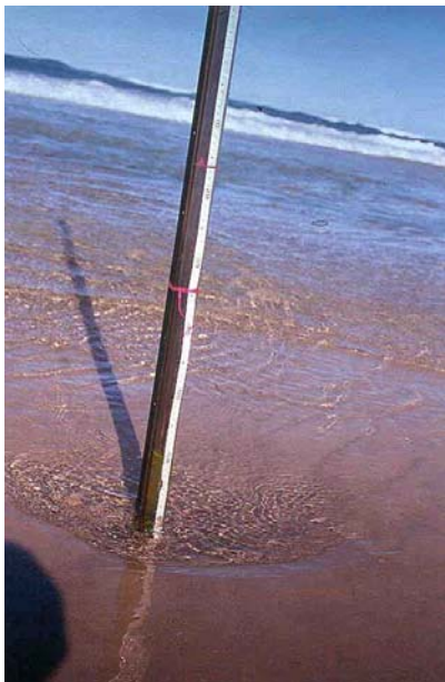
Figure 3.3: Stilling well used to measure the near shore and swash zone mean water level.
