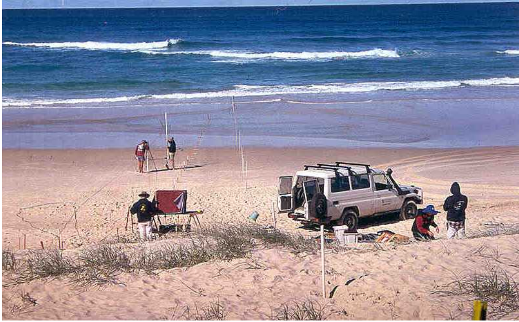
Figure 3.2: Typical field transect (to the right) used to monitor an aquifers response to periodic, ocean forcing. Photo taken of an experiment conducted just south of Point Lookout on North Stradbroke in south-east Queensland.
