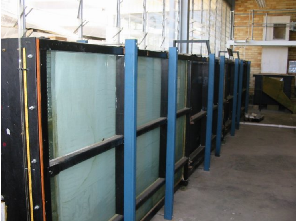
Figure 5.4: The sand flume of dimensions 9m long by 1.5m high by 0.14m wide. The simple harmonic driving head is closest to camera and the far boundary condition is no flow.
