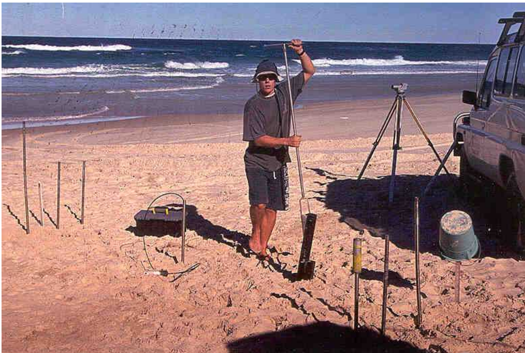
Figure 9.2: Cluster of sampling spears, North Stradbroke Island.
