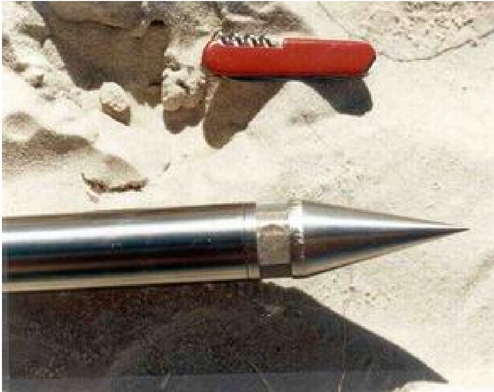
Figure 9.1: Hollow, stainless steel sampling “spears”.
