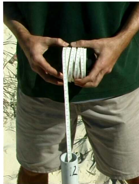
Figure 3.4: Dip meter and piezometer used to monitor subsurface piezometric head levels.
